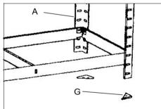
We recommend that the shelving be secured to an adjacent wall using typical wall insert plugs and screws (not supplied) aligned with the slots in the posts.
